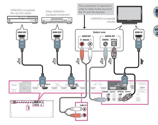
When connecting to an HDMI/DVI-compatible monitor using the HDMI OUT 2 terminal, switch the HDMI output setting to OUT 2 or OUT 1+2. See <u>Switching the HDMI output</u> on page 78.
