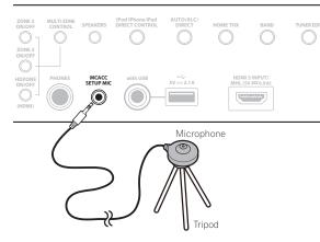
If you have a tripod, use it to place the microphone so that it's about ear level at your normal listening position. If you do not have a tripod, use some other object to install the microphone.
