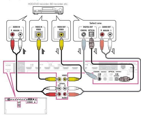
In order to record, you must connect the analog audio cables (the digital connection is for playback only) (page <u>77</u>).
